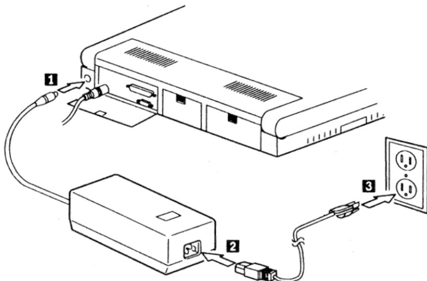
**Note:** If the AC adapter is connected, you can operate the computer even with the rechargeable battery removed. However, if you want to use the AC adapter during Suspend Mode, connect the AC adapter without removing the rechargeable battery.
