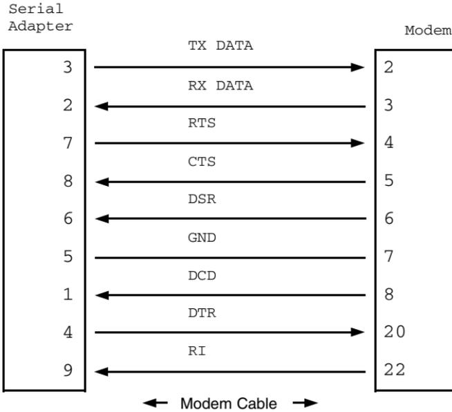
Figure 1. Example of the serial Adapter modem Connection
