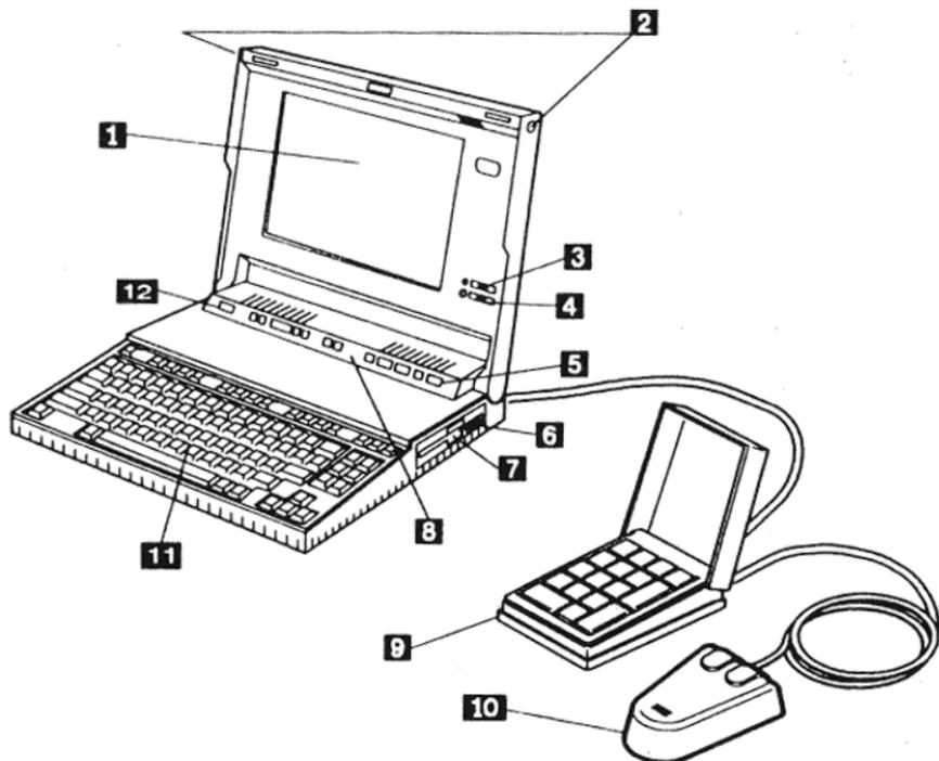
1. **Display (LCD, liquid crystal display)** presents the computer output. You can also use an external PS/2<sup>1</sup> display by connecting it to the external PS/2 display connector at the rear of the computer.
